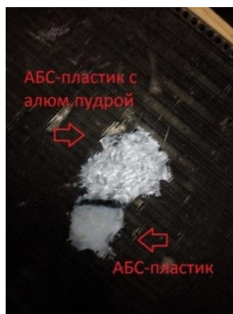
Fig. 2 – Repaired vehicle cooling system radiator
