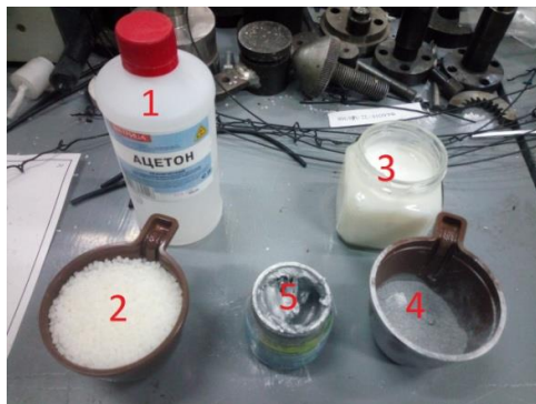
Fig.1 – materials for radiators' repair: 1 – Acetone, 2 – ABS plastic, 3 – Solution of ABS plastic, 4 – Aluminum powder, 5 – Solution of ABS plastic with aluminum powder.
