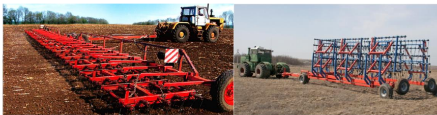
Fig.1 - Spring-tooth harrow at work and transport position
