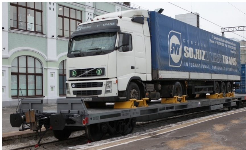
Figure 2 - Piggyback technology of transportation
