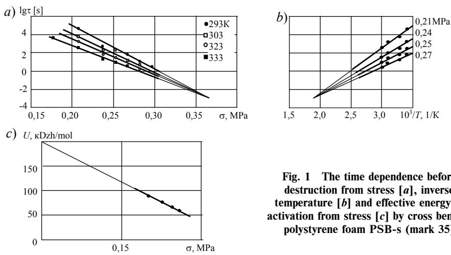
**Fig. 1** The time dependence before destruction from stress [a], inverse temperature [b] and effective energy of activation from stress [c] by cross bend of polystyrene foam PSB-s (mark 35)
