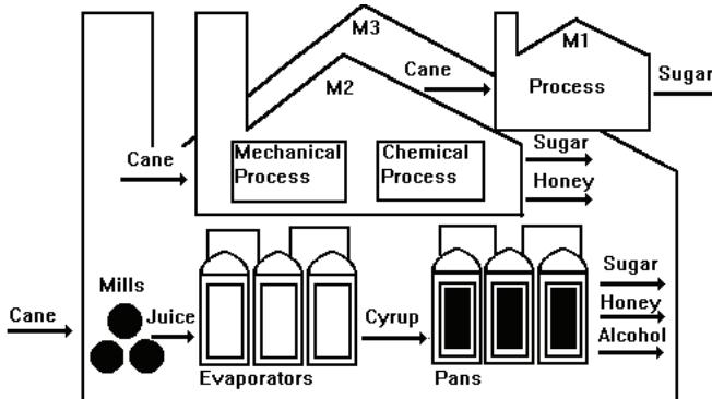
**Fig. 1 Hierarchical multilevel representation of a sugar cane factory**
