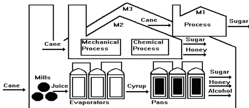
**Fig. 5 Hierarchical multilevel representation of a sugar cane production system**
