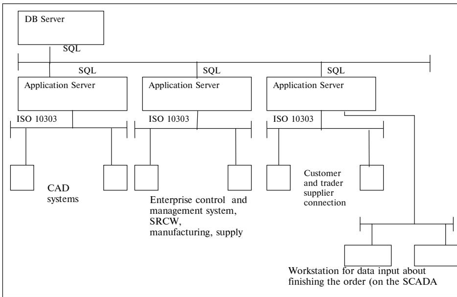
**Fig. 2 Logic structure of a corporate network**
